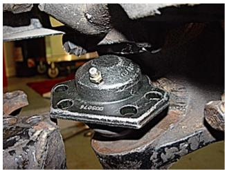
Bend the new joint all the way over to the side. Twist the joint about 90 degrees and it will drop into the hole in the lower geared hub. The first time I tried to put one in I tried to get it in straight and it got caught up and jammed on a small ridge which is part of the geared hub casting. The lower joint goes under the lower control arm.
