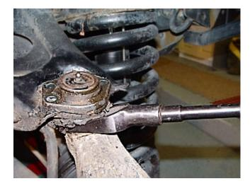
Remove the cotter pin and slotted nut (15/16" socket) from the lower bolt and toss out the old pin. Take a 15/16" ball joint separator (pickle fork) and whack it with a heavy hammer until the ball joint pops up out of the tapered hole. The geared hub will drop down out of the way supported by the lower ball joint.
