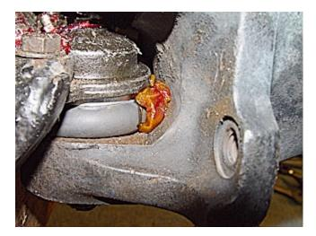
Grease all the ball joints until grease oozes out of the seal. Install your wheels, lower the jacks and you're ready to go. You might want to get your alignment checked.
