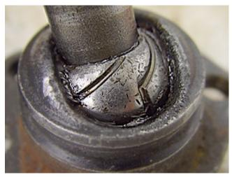
This is a new style upper ball joint. Unlike the older ones this one has grooves on the ball so grease can work it's way to all surfaces of the ball. These ball joints all have grease fittings and can last over 100,000 miles. The one pictured had 58,000 on it.
