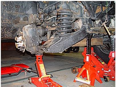
Clean all debris around the hole in the hub and the upper control arm. Drop the new ball joint into the hole in the upper control arm. Make sure that the rubber boot does not get pinched in the control arm hole. Push it down clear through.
