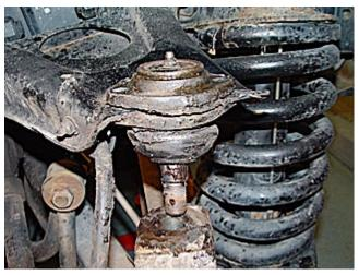
You can now pull the old ball joint up and out of the upper control arm.
