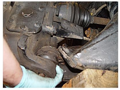
Raise the lower control arm up fairly high (not the geared hub) with a jack and hammer the ball joint till it breaks loose. Jack the arm up a little more and pull the bottom of the geared hub away from the control arm while pulling and rotating the ball joint up and out sideways.
