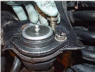
Put a small jack under the geared hub and raise it until the new ball joint bolt is through the upper geared hub hole. Hand tighten the slotted nut.
